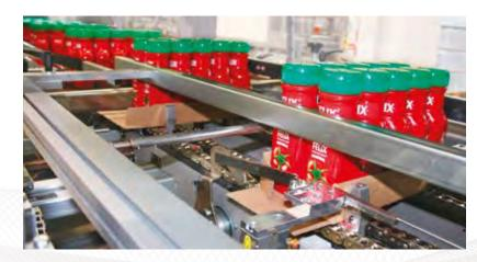
capacity of the container that is being used). Apart from the above mentioned, we have also recently added the CWP ERGON wrap-around case packers, these can produce up to 40 packs/ minute and the new CM FP ERGON combined packer which was designed for packaging in film-only, pad + film, tray + film, tray-only and wrap-around case: all this from a single machine.
