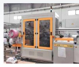
Thanks to a roller belts system, the full pallets are then transferred to the automatic turntable system, which wraps them in wrap-around film.
