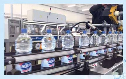
The 12,000 bottles per hour bottling line installed in the plant in Zhdanovichi makes use of a latest generation automation and control system called VaryLine System® that, together with the use of sophisticated sensors, allows you to maintain high levels of operational efficiency throughout the production cycle, thus reducing costs and energy consumption.
