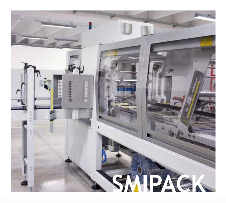
A fter the success of the new range of film shrinkwrappers without sealing bar βP ALX, presented at the end of 2014, SMIPACK has developed the new βP ARX series with the 90° infeed. The new βP ARX packers, which had their world première at IPACK-IMA 2015 in Milan, are especially suited to production needs of up to 20 packs
