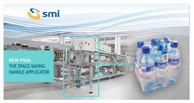
The SK ERGON packers can be equipped with an automatic handle applicator of the **PSHA series** (**Pre-Shrinking Handle Applicator**), which attaches a handle on a section of the shrink film before it's wrapped around a group of containers moving toward the shrink tunnel.
