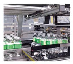
The "Bee-Hive Pack" collation is produced by **Smiflexi shrinkwrappers of the LSK/SK series** and by **Smiflexi wrap-around casepackers of the WP series**, all equipped with a dedicated device arranging containers (bottles or cans) in "staggered" rows in alternate motion and keeping them in that layout all along the whole packing process.
