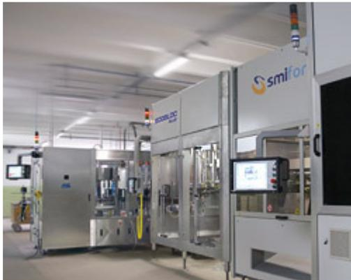
SMI laboratories' relentless engagement in Research and Innovation projects has led to the launch of Smiform's ECOBLOC® PLUS series, featuring integrated systems of **stretch-blowing, filling/capping and labelling** of PET containers with capacity from 0.2 to 3 L, running **up to 36,000 bottles/hour** (depending on the machine model and product features).
