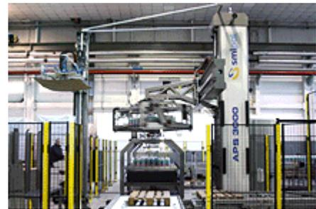
Smipal's palletizers can be easily fitted in any format, product and/or layout change and can provide different types of palletising patterns, according to the customer's specific needs.
