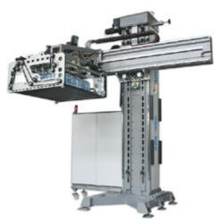
The grip-head picks the pack layers up from a conveyor belt positioned at waist height and, with swift and precise movements, deposits them on the pallet in the desired spot. The beam's vertical motion and the grip-head holding arm's horizontal motion are driven by **brushless motors**, which ensure perfect trajectories during the whole palletisation process. The APS 3000 system's functions can be widened by adding an optional device enabling the grip-head to rotate around its own vertical axe.
