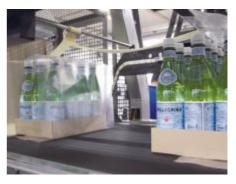
For the automation of the SK 600T shrinkwrapper, SMI has chosen the SERCOS III interface to control the motion axes and to exchange data with the I/O devices mounted on the machine.
