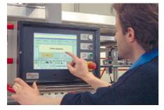
The automatic adjustment device for format change at the machine infeed simplifies the operator's work considerably, as nearly no manual adjustment is required. This turns into **dramatic reduction of the change over time**, enabling quick shifts from a pack size to another, with great benefits to those users who, thank to the SK machines' outstanding versatility, decide to handle many different types of containers in countless packaging configurations.
