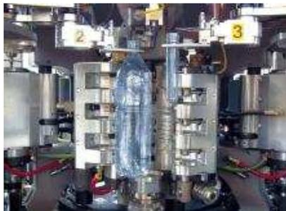
SMI also manufactures **rotary stretch blow molders** for PET, PEN and PP containers up to 36,000 bph. The SR series consists of standard models for the stretch-blow moulding of bottles from 0.25 to 3 litres and SR HC -High Capacity models for bottles from 3.5 to 10 litres.
