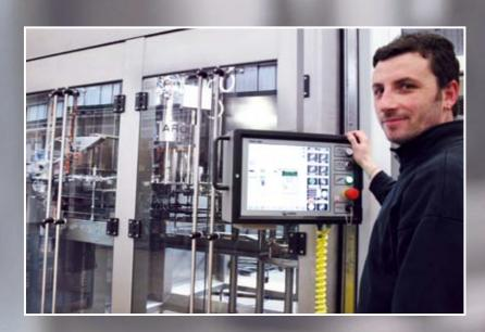
The primary packaging of Antigua Distillery's Oasis mineral water in 0.35 litre, 0.65 litre and 1.5 litre PET bottles is performed by Smiform's stretch-blow moulding, filling/capping ECOBLOC® 4-28-8 LG-VMAG integrated system, while the secondary packaging in shrink film packs with and without flat cardboard pad is performed by a Smiflexi LSK 25 P model shrinkwrapper.
