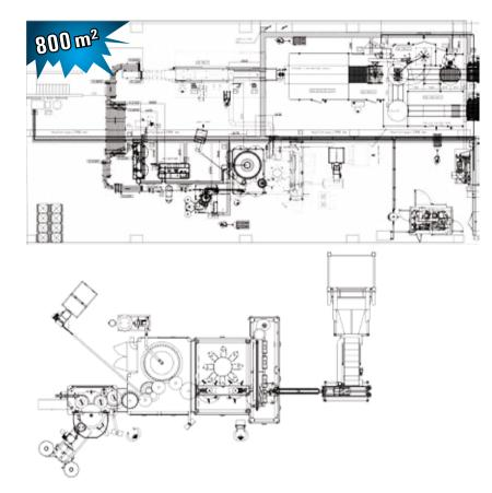
The secondary packaging unit, designed by SMI from scratch, is an innovative shrink film packaging system which includes thrust integration between the shrinkwrapper and the palletiser; this solution has allowed for the area occupied by the end of line machines to be contained and involves a drastic reduction in connecting conveyors between the shrinkwrapper and palletiser;
