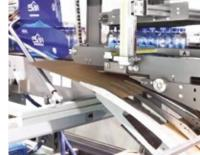
The proposed solution includes an integrated system of the ECOBLOC® ERGON range for stretch-blow moulding, filling and capping operations of PET bottles combined with a wrap-around case packer for secondary packaging of the LWP ERGON range and an APS ERGON palletiser.
