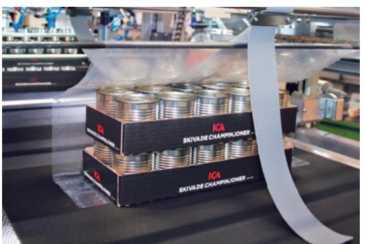
other types of plastic, glass, metal and cardboard containers in packs in film only, in cardboard pad + film or in corrugated cardboard tray + film. The available models enable to automate the secondary packaging process within production plants from 30 up to 45 pack/minute (the second figure refers to film only in triple lane).
