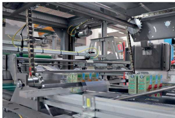
picker equipped with a group of suction cups with pneumatic vacuum system run along the cardboard ramp and are positioned under a group of incoming products with the long side leading
