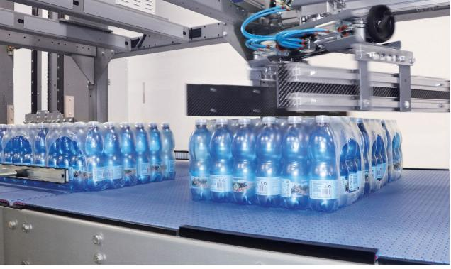
motors, which guarantee perfect trajectories during all palletising phases. All the operations are managed by a "user-friendly" machine, automation and control system, which allows the operator to use the palletising system easily and efficiently.
