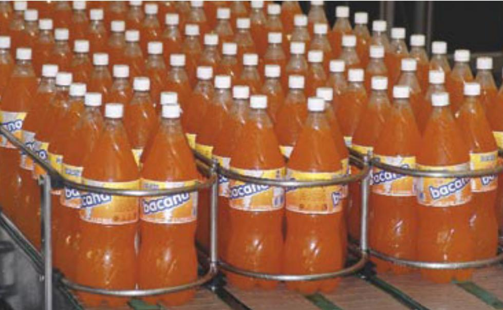
2 litre PET bottles in 3x2 shrink film packs. The machine is also, however, able to package other types of containers already used by the Brazilian company, such as aluminium cans.
