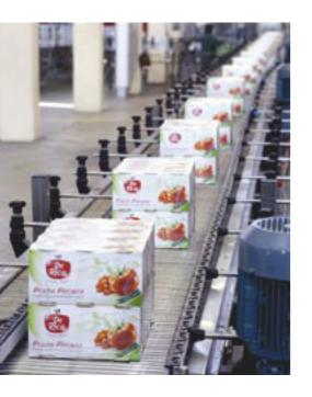
flexibility, guaranteed by the presence of machines with high technological content such as the Smiflexi SK 600T shrinkwrapper, equipped with tray stacker, and the Smiflexi MP 300 sleeve packer.
