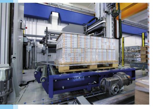
Smipal, a SMI division specialised in the production of automatic palletising systems, offers reliable cuttingedge solutions with the APS P series. The APS P model features a SCARA arm and integrates in its central column the operations of palletising, empty pallet feeding and pad insertion - three different operations usually performed by separate machines inside their own dedicated space.
