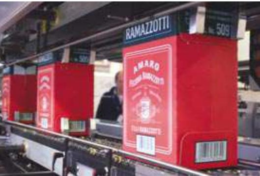
bottles with differing capacities (from 0,375 to 1,5 litres) are in fact grouped into formats of 2x3 and 3x4 and then packaged in wrap-around boxes with and without the insertion of preformed board partitions.
