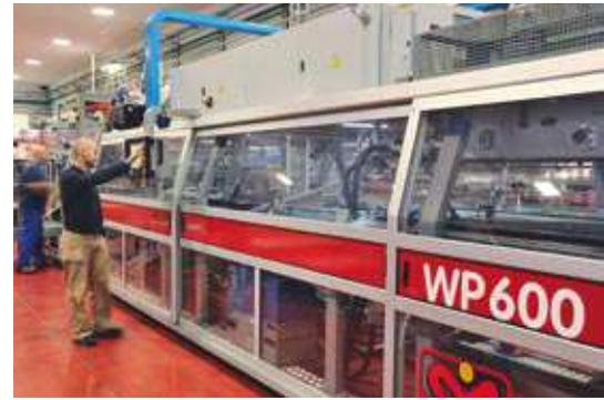
The process of inserting the partitions and loading the relevant magazine is also faster, as these are already pre-assembled. The size of the casepacker remains the same as that of a standard machine, as both the partition magazine and the insertion device are assembled in the upper part of the frame of the packaging machine.
