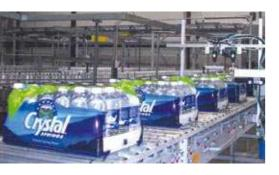
package the PET bottles of 0.5 litres in 4x3 formats, film only in a double lane.
