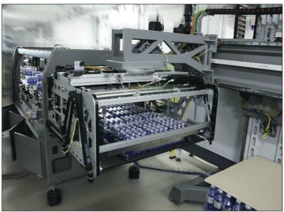
gripping head by a motorised bars system. The infeed with the continuous in-line pre-composition is very compact and reliable and stands out from traditional ones for its one-way motion and for the possibility of orienting the bundles in any position.
