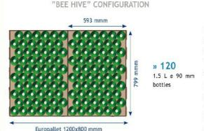
The collation is produced by Smiflexi shrinkwrappers of the LSK/SK series and by Smiflexi wrap-around casepackers of the WP series, all equipped with a dedicated device arranging containers in staggered rows in alternate motion and keeping them in that layout all along the whole packing process.
