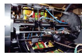
6 oz. tinplate cans in 1x3 and 1x2 collations. The machine chosen by Hida is very versatile and can also pack bottles, cartons and plastic, metal and glass jars in various types of pack at speeds up to 300 pack/minute (depending on the type of container and format selected).
