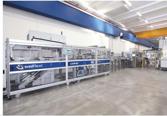
and uninterruptedly, by an innovative up-going, slightly curved system that significantly improves continuity in the feeding of the packaging material. Smiflexi's LWP series new wrap-around case packers have a compact and solid frame, able to adapt easily to any logistic condition and also mount brushless motors that drive the axes, which allows the user to reduce energy consumption.
