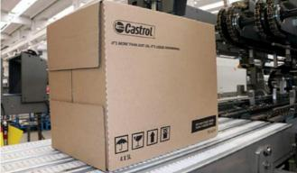
are the solutions supplied by SMI for the secondary packaging of 5L jerrycans of lubricating oil in wrap-around boxes.
