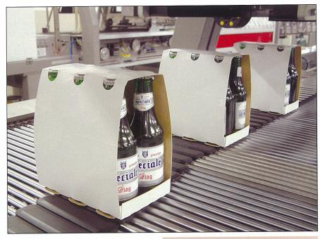
The pack collations can vary according to the containers shape and dimensions; in general, the most widespread collations are: 1x3, 1x4, 2x2, 2x3 and 2x4. All MP models feature an electronic grouping system; the change-over is manual.
