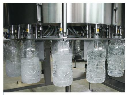
module and the wet environment of the filling/capping module. Excellent quality/price ratio, environmental performance, low TCO and reduced maintenance make of ECOBLOC®PLUS the ideal solution to blow, fill, cap and label PET containers with up to 3 litres capacity, running up to 36,000 bph (depending on the machine model and product features).
