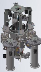
4-cavity versions, and offer all the advantages of rotary technology in a "speed" range (1,000 to 9,200 bottles/hour), traditionally served by linear stretchblow moulders. In fact, due to advanced technological solutions, the ERGON EBS K range is capable of producing PET containers up to 3L, with output up to 2,300 bottles/hour per cavity for 0,5 L formats. The new SMI compact stretch-blow moulder offers a long list of advantages that make it stand out in its market:
