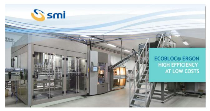
The integrated plants of the new **ECOBLOC® ERGON** series are the ideal solution for the **blow-molding, filling and capping of PET and PP containers** for the bottling of **still and carbonated water, soft drinks, milk and edible oil** up to 3 L at the maximum output of 33,600 bottles/hour (0.5 L). The series includes also High-Capacity models (ECOBLOC® HC) for containers up to 10 L and maximum output of 7,200 bottles/hour (5 L).
