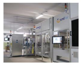
SMI laboratories' relentless engagement in Research and Innovation projects has led to the launch of Smiform's ECOBLOC® PLUS series, featuring integrated systems of **stretch-blowing**, **filling/capping and labelling** of PET containers with capacity from 0.2 to 3 L, running **up to 36,000 bottles/hour** (depending on the machine model and product features).
