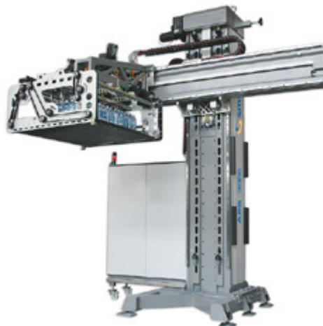
The grip-head picks the pack layers up from a conveyor belt positioned at waist height and, with swift and precise movements, deposits them on the pallet in the desired spot. The beam's vertical motion and the grip-head holding arm's horizontal motion are driven by **brushless motors**, which ensure perfect trajectories during the whole palletisation process. The APS 3000 system's functions can be widened by adding an optional device enabling the grip-head to rotate around its own vertical axis.
