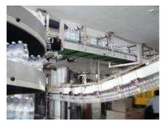
Empty PET containers are quickly and trouble-free transferred from the blow molder to the filler.
