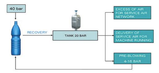
The new air recovery system, installed as standard equipment in all SMI blow molders, grants:
