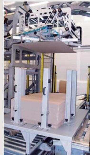
The vertical axis is made up of a fixed column along which the horizontal beam slides on guides with recirculating ball bearings.
