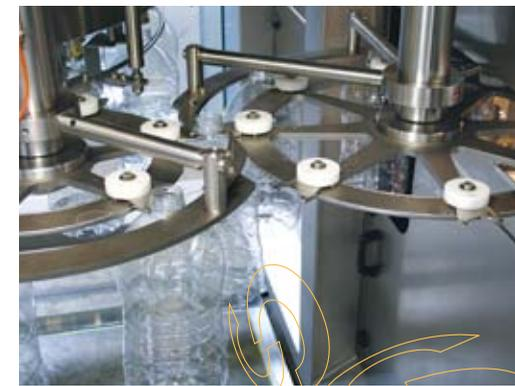
Smiform's integrated system installed in the facility of Pinar Su produces 3.25 litre and 5 litre PET containers at the speed of 6,000 bph and 10 litre containers at 4,200 bph.
