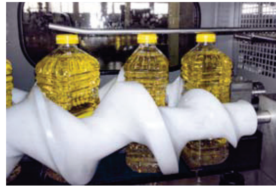
Above: the new device at DV500 inlet is designed to orient the bottles with the handle in the required position.
