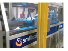
plant manufacturing in for Smyrna, Tennessee, which SMI has provided Vi-Jon with a series of machines for the Rubbing Alcohol packaging line. Specifically, the new of a supply consists Smiflexi model WP 350 wraparound case packer for secondary packaging in cardboard boxes, a DV
