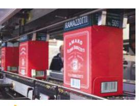
bottles with differing capacities (from 0,375 to 1,5 litres) are in fact grouped into formats of 2x3 and 3x4 and then packaged in wrap-around boxes with and without the insertion of preformed board partitions.
