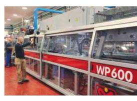
The process of inserting the partitions and loading the relevant magazine is also faster, as these are already pre-assembled. The size of the casepacker remains the same as that of a standard machine, as both the partition magazine and the insertion device are assembled in the upper part of the frame of the packaging machine.
