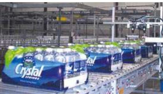
package the PET bottles of 0.5 litres in 4x3 formats, film only in a double lane.
