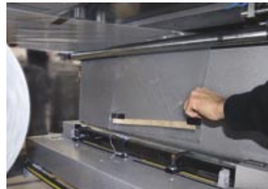
The splicing operation occurs without the need to stop the packaging process.
