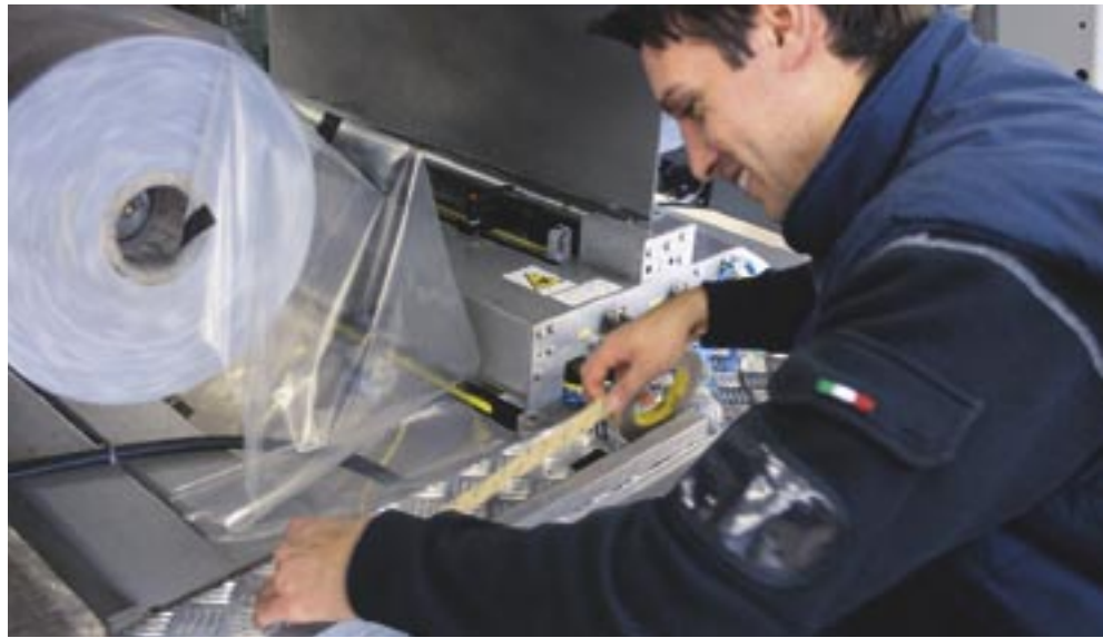
reels of shrink film installed beneath the work surface of the machine.
