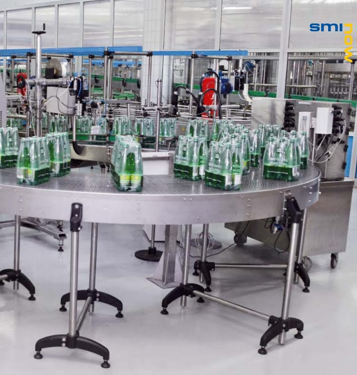
and glass (0.355-liter, 0.75-liter and 1.0-liter bottles) in wrap-around cardboard boxes with and without the preformed cardboard separators. More specifically, the 0.5-liter PET bottles are packed in the 4x6 configuration, while the 1-liter bottles in the 3x4 collation are packed in wrap-around boxes with and without separators.
