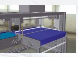
The APS 1550 P PLUS palletizing system satisfies production requirements up to 50 packs per minute (about 150 layers per hour) and can handle 800x1200 mm (europallets) and 1000x1200 mm pallets.
