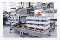
Furthermore, the integration of multiple functions (all housed in one central column) offers considerable advantages as far as operative flexibility, workplace safety and machine maintenance are concerned. Another advantage of the compact design of the APS PLUS systems is the option of concentrating the use of forklifts, transpallets, etc. in a well-defined zone, optimizing the management of the loading and unloading areas.
