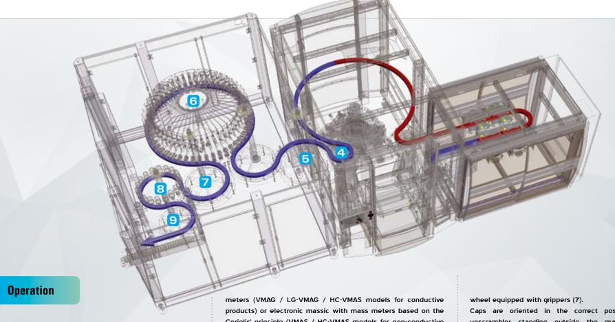
The bottles are conveyed directly from the blower to the filler neck-handling style by means of transfer star-wheels.
